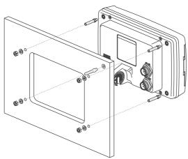
Figure 2.2 - Example of Flush installation CPF180i
